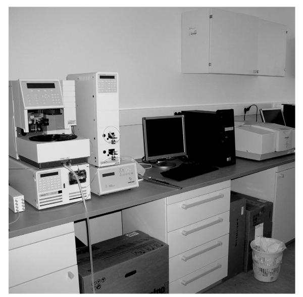
HPLC and IR-Spectrometer devices
