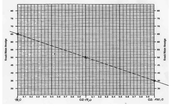
Diagram for the calculation of octane rating
