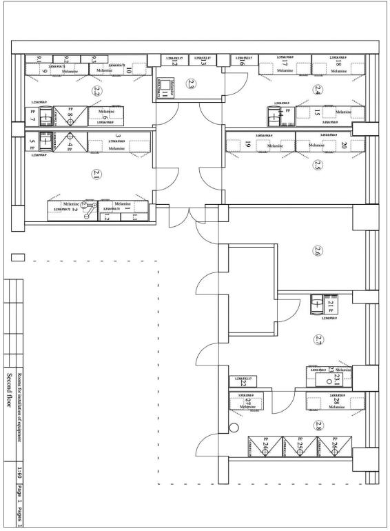
3.2.1.1 Floor plan of the laboratory inclusive sinks and exhausters
