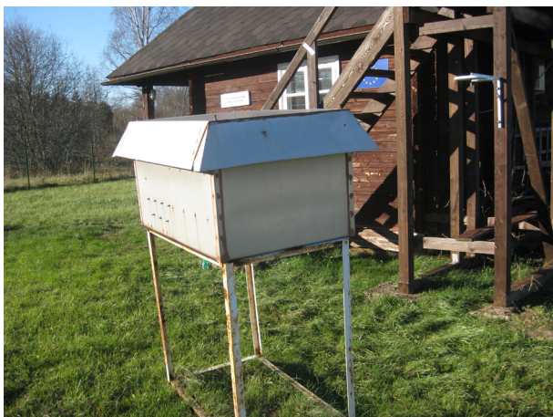
Fig. 1. Lahemaa corrosion observatin station (a), passive samplers for HNO 3 and particulate matter protected from wind and precipitation (b), a carousel on which rock samples are attached (c), materials plates exposed to the weather (d), and box for investigating the soiling of modern glass (e).
